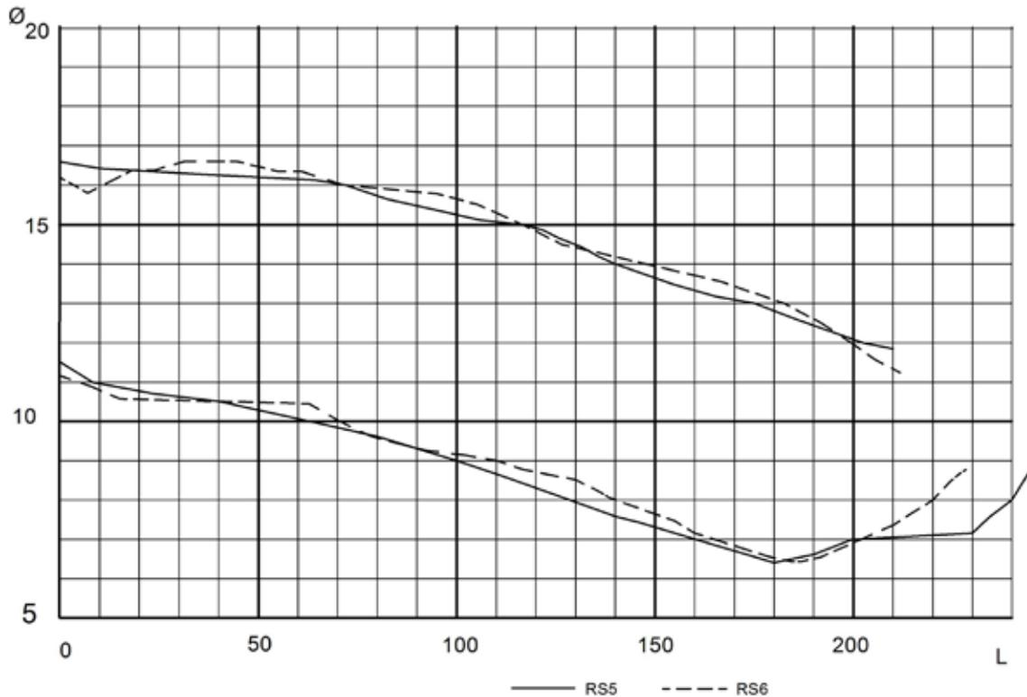
Fig 12: bore profiles of RS5 and RS6
