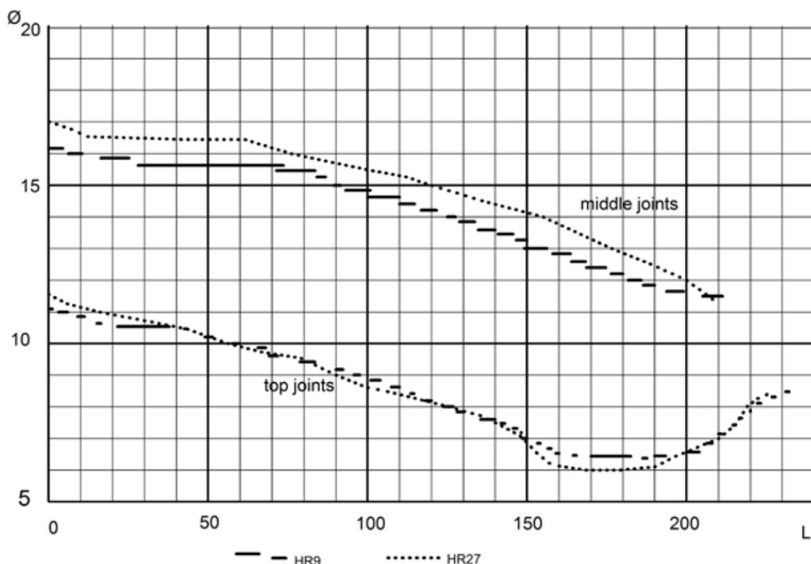
Fig. 7: The bore profiles of HR9 and HR27. The joints of HR9 are on cross section rather oval, the lines in the graphic connect the minimum and maximum depth (length) for each of the bore gauges (which were used with diameter steps of 0.2 mm).
