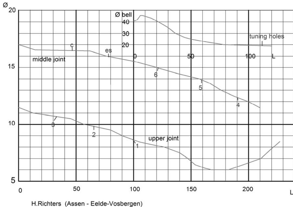
*In these graphs the bore dimensions of upper and middle joint are drawn in a scale of 10:1 to the length of these joints.\* The bore of the bell is drawn in a scale of 1:1 (diameter to length). All diameters are related to the lower end of each joint (= 0 in the length scale). The toneholes are indicated with 1 to 6, the keyholes with es (=e-flat, or d#) and C.*
