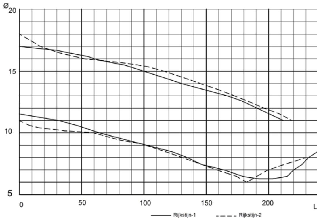
Fig. 13: bore profiles of two oboes by Rijkstijn
