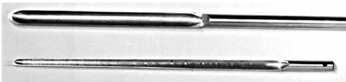
*Figure 3: modern reamers for woodwind instruments, from the website of the firm of Joseph Böhm (Germany). These reamers are made on a modern computerized metal lathe.*
