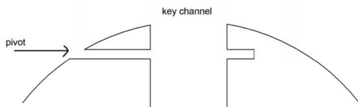
As the pivots hardly protrude from the holes, no attempt was made to remove them. That means that I could not assess exactly the size and shape of the key holes and the key channels. The material of the key springs could not be assessed as well; but it is clear that - as on the other oboes of Hendrik Richters - the springs are attached (shoven) in the key channels. The key pads are made of a felt-like material; it was not possible to assess whether these pads are original.
