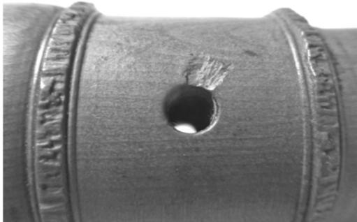
*The waist of the bell with resonance holes and 'nibble damage' at the beads.*
