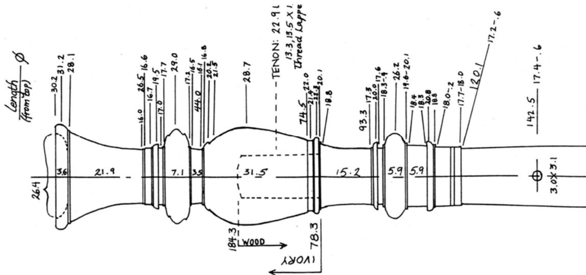
*Measurements of the baluster of the oboe 2037 by Hendrik Richters (Bate Collection, Oxford, drawing by Dick Earle, 1989)*
