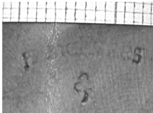
Notes: \*Comparing makers' marks from different instruments is not easy, measuring their dimensions on curved surfaces is tricky. The best way is to do all your measurements yourself, using the same method (for instance using graph paper - see photo - instead of callipers for assessing the length of the stamps).
